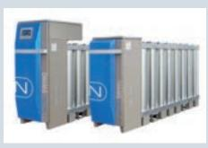
For large production capacities, a "Dual Bank" can be added consisting of a second PSA nitrogen generator without any PLC or power supply. The Master Dual Bank gets its power and control signals from the NITROSWING\* PSA nitrogen generator through a single cable connection, with one master NITROSWING\* PSA nitrogen generator controlling up to three Dual Banks simultaneously.
